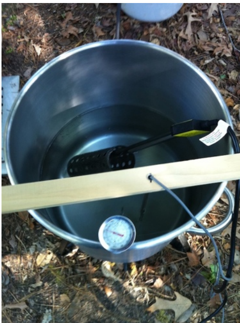
Picture 4 - Close-up of water heater, thermometer and temperature probe in kettle for sparge water temperature hold test
