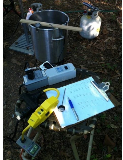
Picture 5 – Overall setup for sparge water temperature hold test
