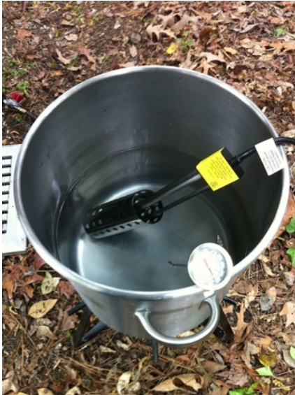
Picture 2 - Water heater placed in kettle for heat performance test
