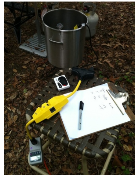
Picture 3 - Overall setup for heat performance test (note the GFI circuit included in the setup for safety)
